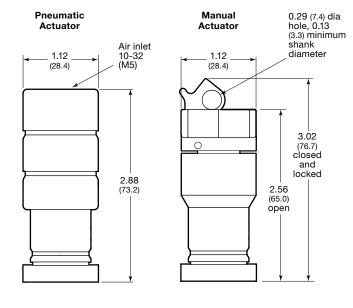
Dimensions shown for standard manual and pneumatic actuators. Contact your authorized Swagelok representative for dimensions with optional actuators.
