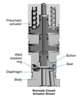
Wetted components listed in *italics*. Actuator component materials shown for standard manual and pneumatic actuators; contact your authorized Swagelok sales and service representative for optional actuator additional materials.
