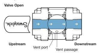
When the valve is closed, shutoff occurs only on the downstream side. Upstream fluids flow through the vent passage to the vent port and are released to atmosphere.
